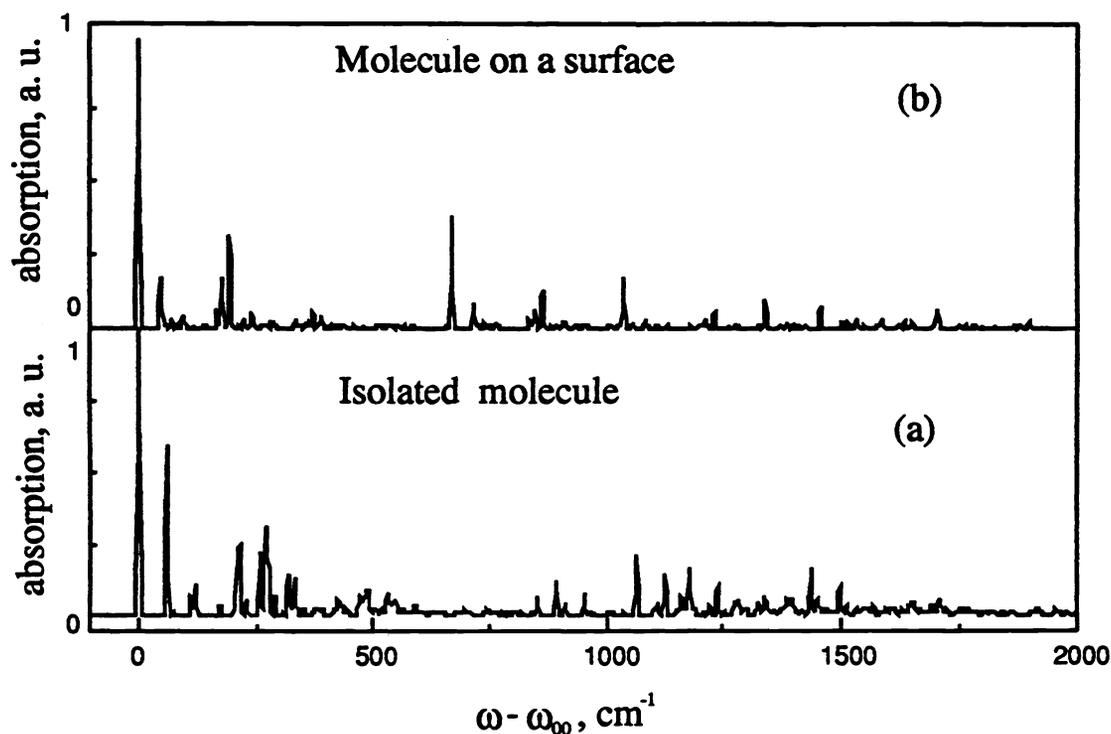
Figure 2: Calculated absorption spectra of (a) isolated and (b) surface-adsorbed *trans*-stilbene.
