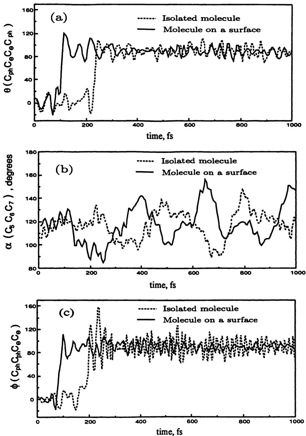
Figure 3: Time dependence of (a) torsional angle  $\theta(C_{ph}C_eC_eC_{ph})$ , (b) bending angle  $\alpha(C_5C_6C_7)$  and (c) phenyl twist angle  $\phi(C_{ph}C_{ph}C_eC_e)$  calculated along a representative single MD trajectory *cis*-stilbene ( $\pm 180^\circ$  angles are geometrically identical).
