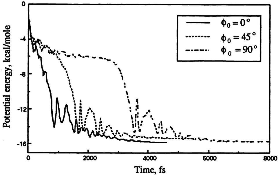
Figure 1: Calculation of the equilibrium state of *cis*-stilbene molecule on the surface. Time dependence of the molecule's potential energy. Damping rate is equal to 1 ps,  $\phi$  is an orientation angle with respect to the surface.
