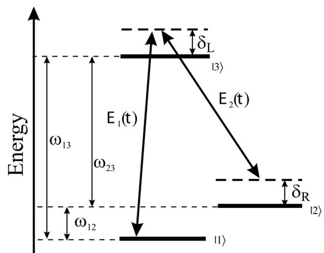
**Fig. 1**  $\Lambda$ -system driven by two laser fields  $E_1(t)$  and  $E_2(t)$ . Here  $\delta_L$  is the one-photon laser detuning at the transition  $|1\rangle \leftrightarrow |3\rangle$  and  $\delta_R$  is the two-photon Raman detuning
