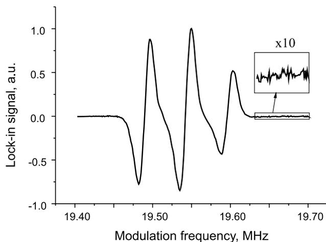
**Fig. 11** Spectrum of the dark resonances taken from a vapor of Rb atoms in a buffer gas at the constant magnetic field. All resonances are split into three components due to the quadratic Zeeman effect. The magnetic field induction was roughly 14 G, the power of the pumping laser field  $P = 140$   $\mu\text{W}$ , and the synchronous detector time constant  $\tau = 3$  ms
