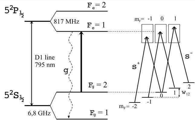
**Fig. 2** Structure of the  $D_1$  line in  $^{87}\text{Rb}$  atom. The levels of the working transition  $F_g = 2 \rightarrow F_e = 1$  are split in the applied magnetic field into  $2F + 1$  sublevels each. The pairs of Zeeman sublevels of the ground state  $\Delta m_F = 2$  and those of excited state form a chain of three  $\Lambda$ -systems
