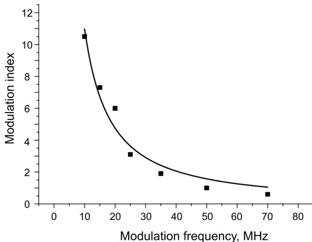
**Fig. 8** Typical dependence of the FM modulation index  $M$  of the semiconductor laser radiation vs the modulation frequency  $\Omega_{\text{mod}}$ . The amplitude of the generator voltage, which creates modulation of the laser diode current, was maintained constant. Solid line shows approximation by the function  $M = A/(\Omega_{\text{mod}}/(2\pi \times 1 \text{ MHz}))^B$ , where  $A = 1.7(6) \times 10^2$  and  $B = 1.21(14)$  are the approximation parameters
